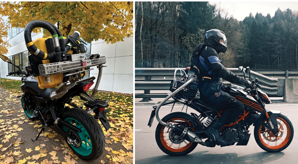
Vehicles with mounted on-road measurement equipment. Left a category L3e-A3 motorcycle with standard PEMS. © TU Graz/AIP GmbH Right a category Le3-A1 motorcycle with a SEMS. © TU Graz/Horiba
