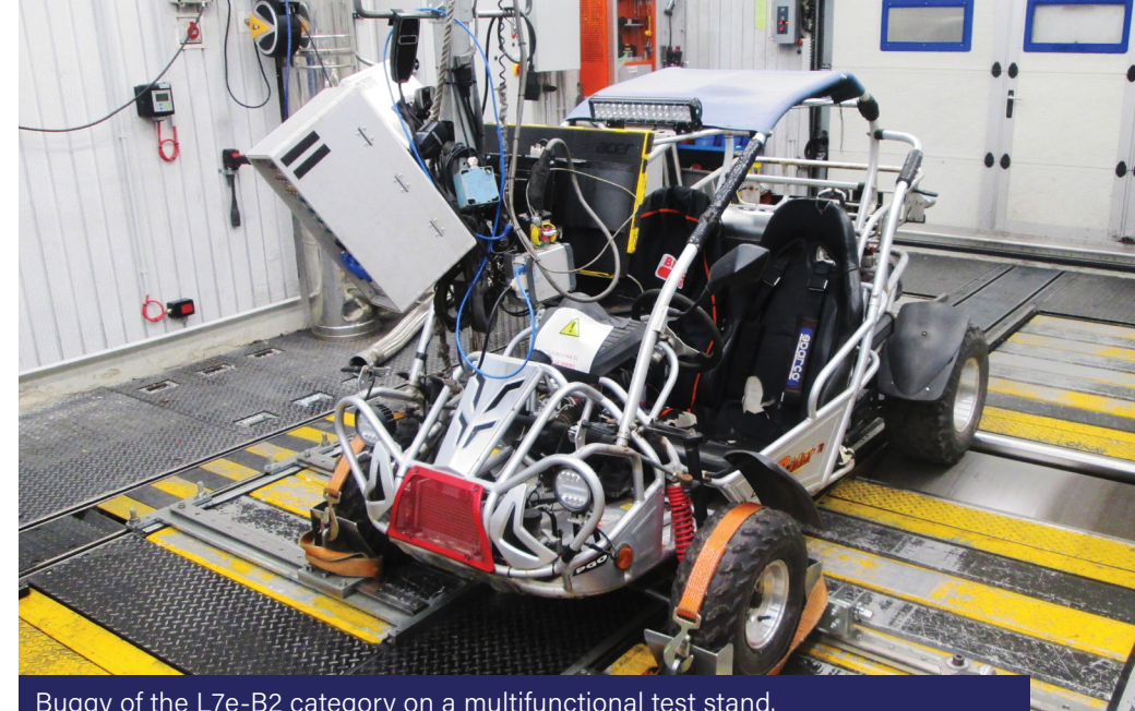
Buggy of the L7e-B2 category on a multifunctional test stand.
