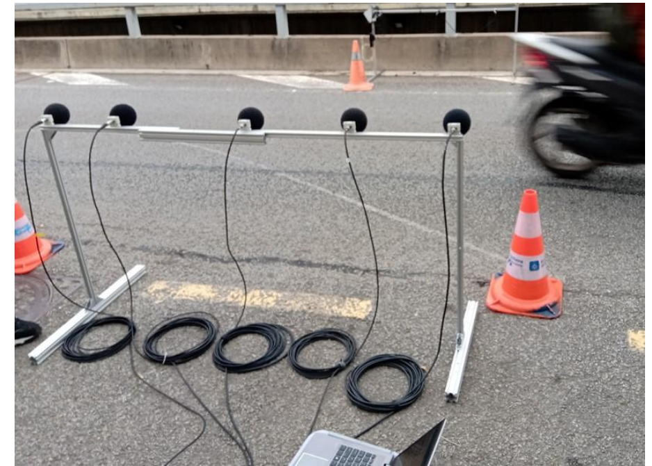
KU Leuven microphone array noise measurement system
