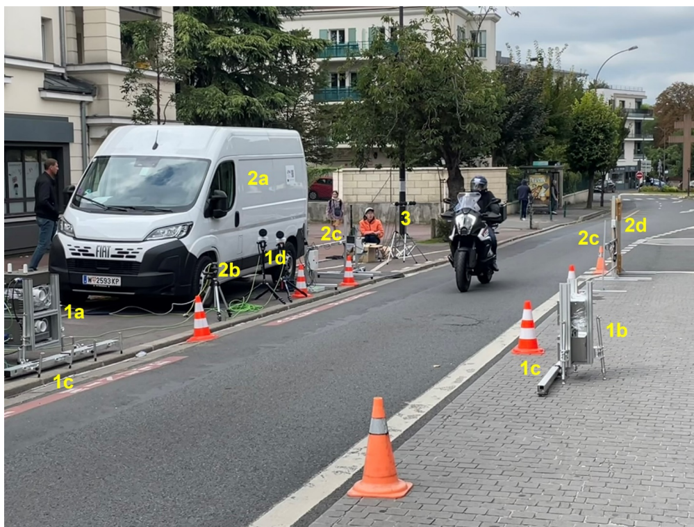
Figure 8. Typical instrumental set up in the LENS tampering in-field survey: 1. Opus RSD 6000 dual remote sensing system: 1a. source/detector module, 1b. lateral reflective mirror, 1c. speed and acceleration measurement bars, 1d. automatic license plate readers; 2. TU Graz point sampling system: 2a. van hosting measurement instruments for PN, BC, NO x and CO 2 , 2b. air sampling inlet to instruments in the van, 2c. stands for triggering of passing vehicles and Schlieren imaging; 3. KUL array of noise measurement microphones.
