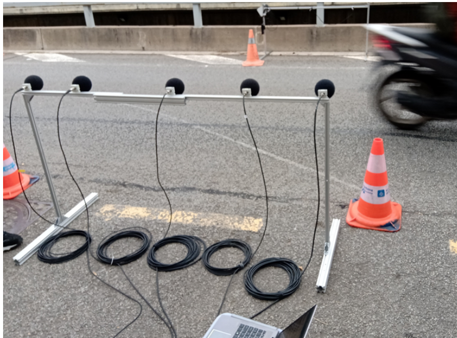
Figure 7. Picture of the microphone array used in the Barcelona campaign. A similar setup, mounted slightly higher, was used in the other campaign.
