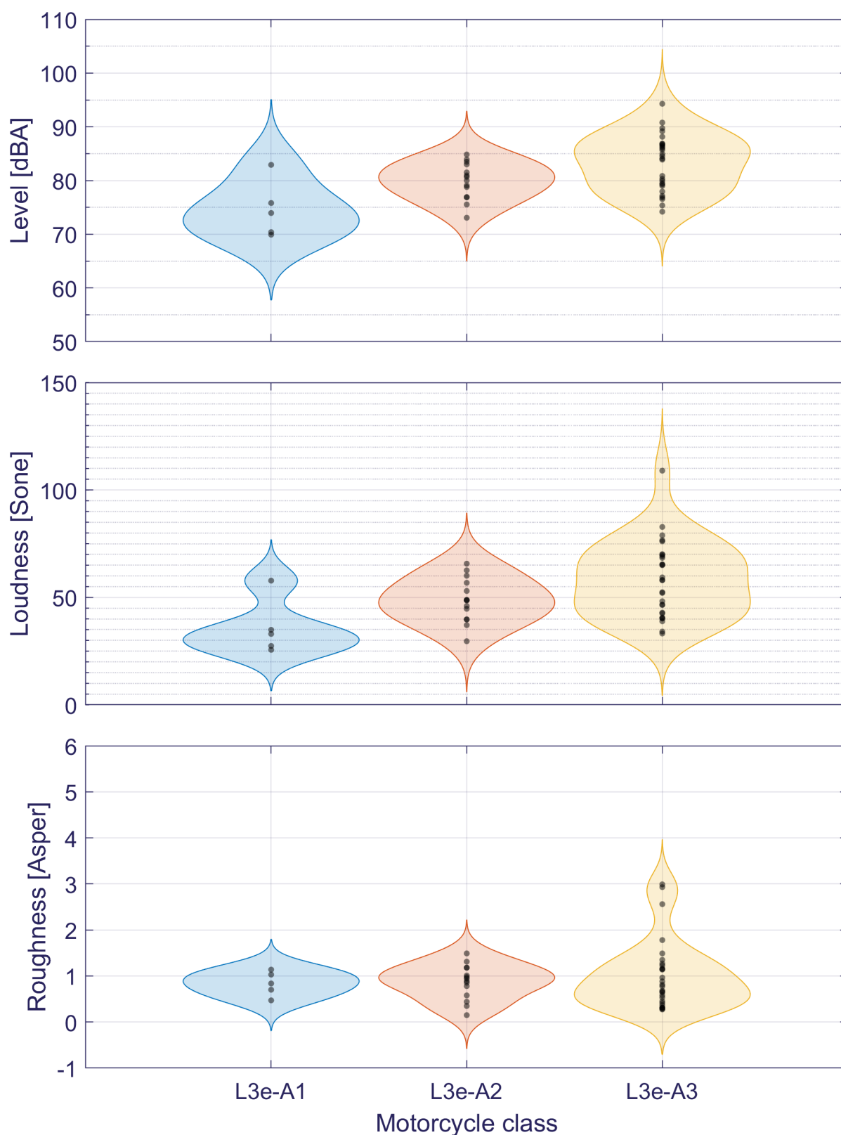
Figure 3-22: Acoustic parameters vs. subcategory for driving pattern 11 (gear shift, from const. speed, gear 3 to 2)
