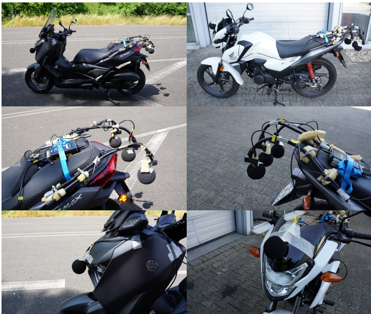
Figure 4-1: Microphone setup (three in the back, one in the front) on the vehicles V1 (left) and V2 (right)
