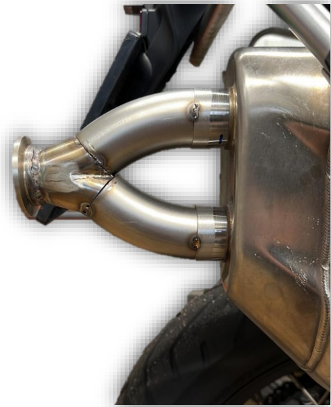
Figure 3-1: Example of cone fitting for exhaust gas flow measurement device and tail pipe connection in a double tail pipe configuration
